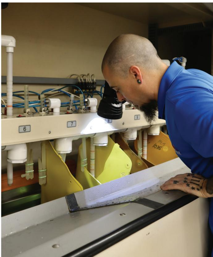
Jake Lawler, CESI lead lab technician, checks water levels of the machine before gloves are tested. Photo by Carli Eubank.
