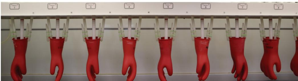
Gloves are clipped and ready to be machine tested after being visually inspected by employees for any cuts, tears, ozone or other damages to the material. In 2022, CESI employees retested 64,644 gloves. Photo by Carli Eubank.
