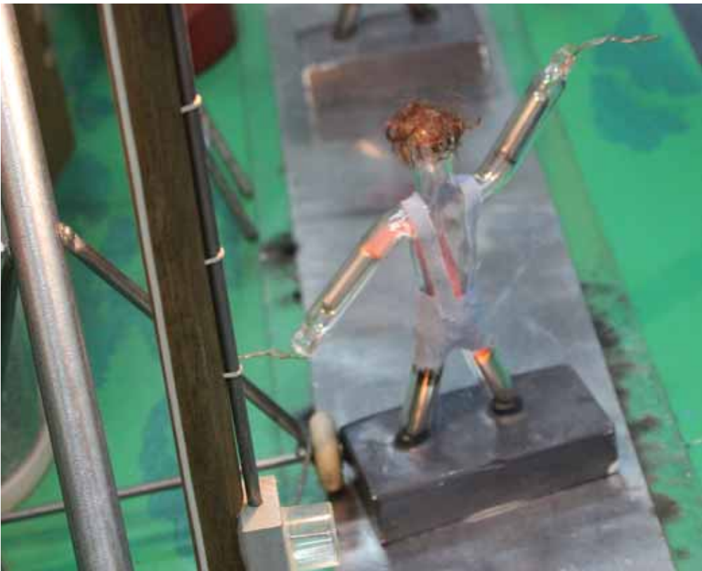
Neon Leon’s body is made of glass fuse tubes. When he “touches” an object that is energized, such as a grain auger leaning against a high voltage power line, Leon lights up in bright orange, as shown above. Mike Stephens, power use adviser for Cotton Electric, recently used Electric Junction, where Neon Leon and Lightnin’ Liz “live,” to demonstrate safe practices around electricity.
