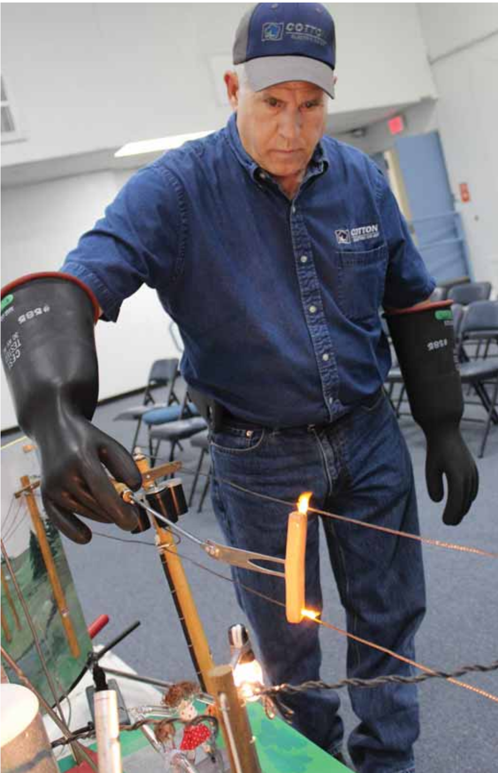
Mike Stephens holds an ordinary frankfurter between an energized and neutral line to demonstrate how electricity can pass through a human body.
