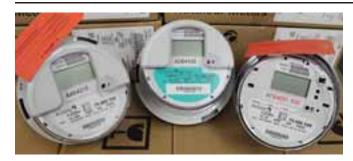
Aclara meters are recording power use at all residential and most commercial locations served by the Randlett substation. All Cotton Electric meters are labeled with unique identifying numbers. Numbers on Aclara meters are prefixed either with AA, AD or AC.
