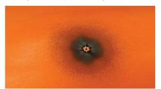
A testing machine identified a punctured hole in a blanket, burning a hole all the way through the failed equipment. Photo by Carli Eubank.
