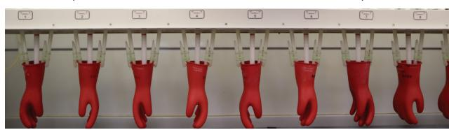
Gloves are clipped and ready to be machine tested after being visually inspected by employees for any cuts, tears, ozone or other damages to the material. In 2022, CESI employees retested 64,644 gloves. Photo by Carli Eubank.
