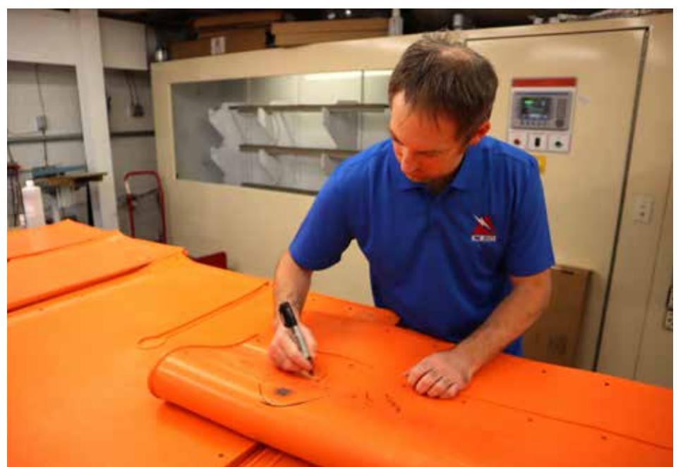
Cotton Electric Services Inc. Lab Technician Ryan Noland marks a rubber blanket that failed during electric testing. Photo by Carli Eubank.
